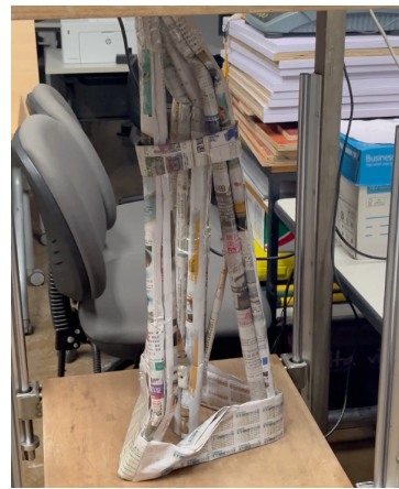
(b) Immediately after failure
